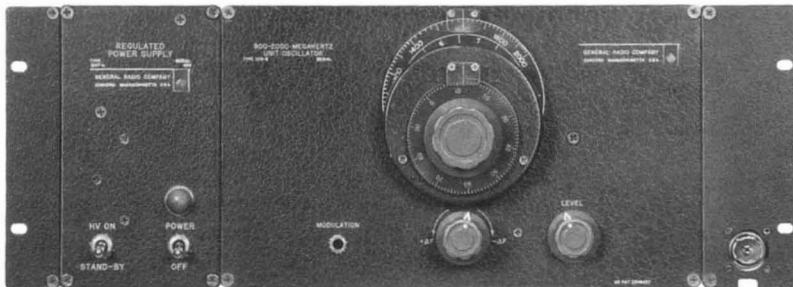
Figure 2-1. Type 1218-B7R rack-mounted rf source, typical of the wide variety of rack-mount oscillator/power-supply combinations available. A special coaxial patch cord supplied brings oscillator rf output to the GR874 connector shown at right. Rack height is 7 inches.
